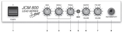
\*NOTE: The JCM-1H front panel is illustrated. The JCM-1C panel is identical but runs in the opposite direction.
